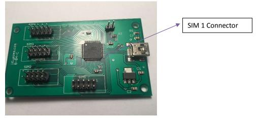
Each Sim Connector is labeled on the Board. There are 4 Sim Connectors labeled SIM 1, SIM 2, SIM 3 and SIM 4.
